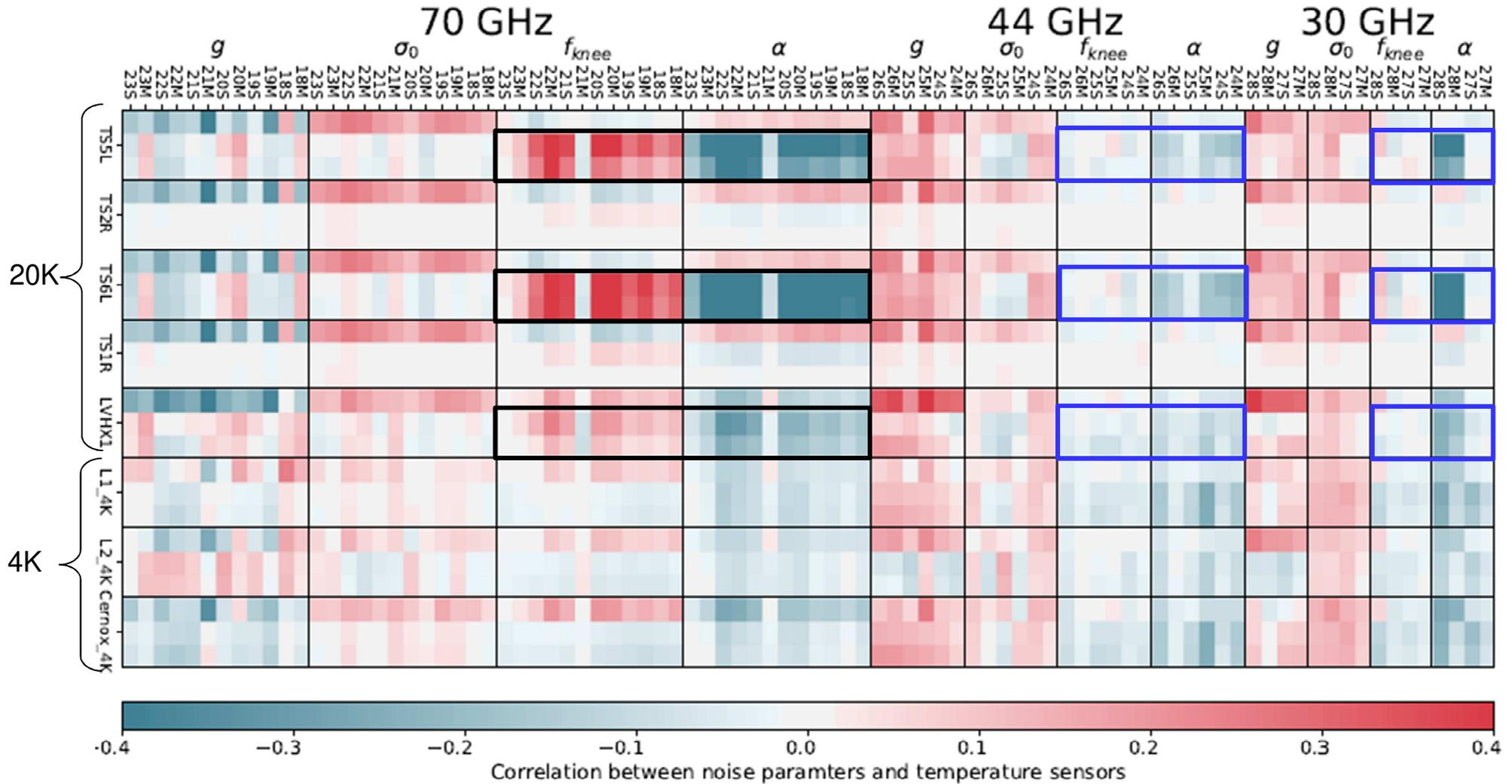
**70 GHz:** rms and p-p of  $T_{20K}$  correlate with  $f_{knee}$  and anti-correlate  $\alpha$  (*steeper spectrum*)
