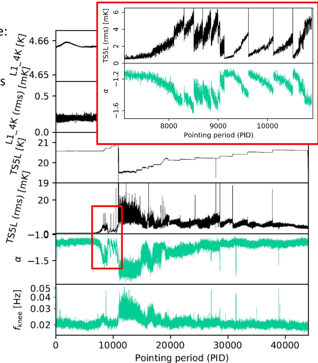
Strong correlation between  $T_{20K}$  fluctuations (rms) and 70GHz  $\alpha$ ,  $f_{knee}$
